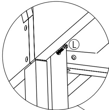
Screws to attach the expansion and second back leg comes with the expansion kit DSF265
